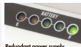
Redundant power supply (Charging of the battery is approximately 8 hours)
